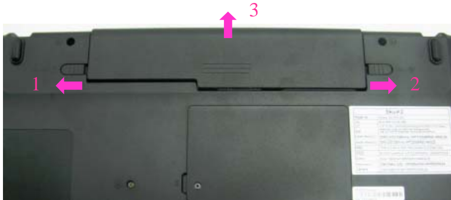
Figure 4-1 Removing the battery pack
