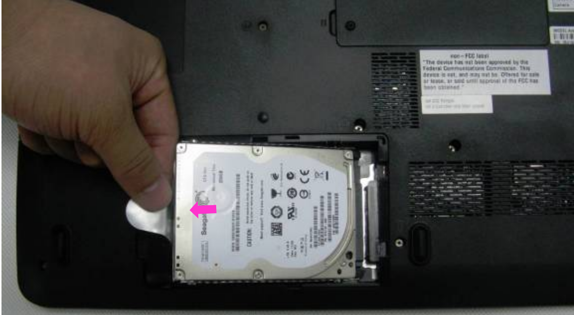
Figure 4-4 Removing the HDD assembly
