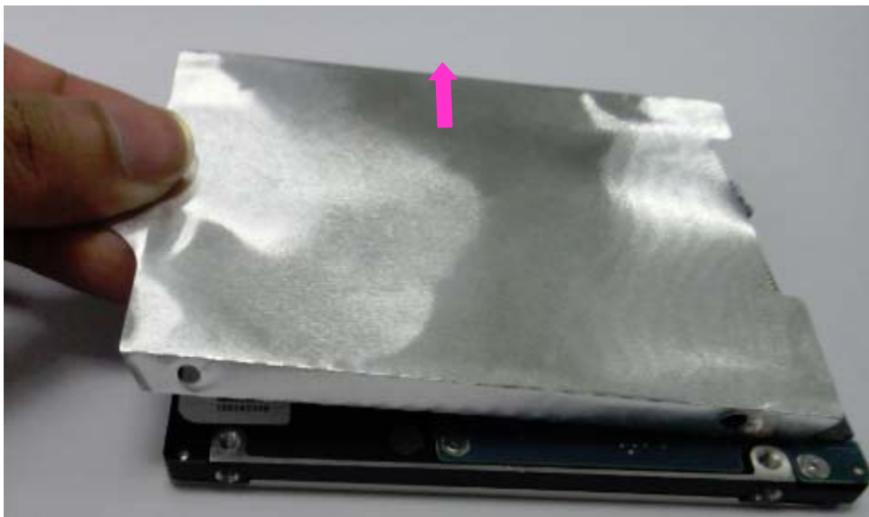
Figure 4-5 Separating the HDD and HDD Mylar
