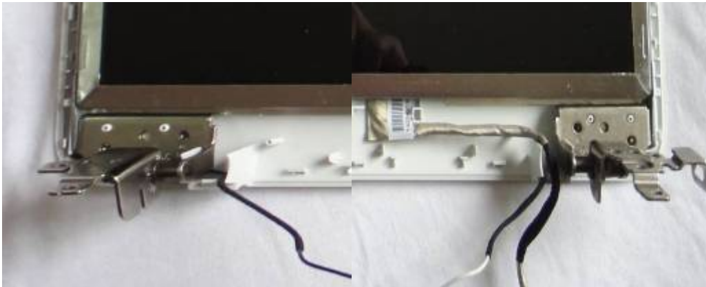
Figure 4-34 Removing the LCD Unit
